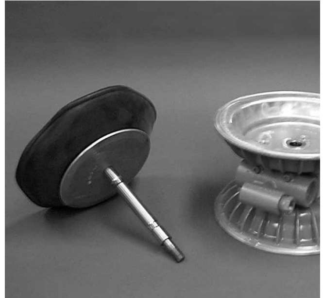
Step 9A. Figure 9A NOTE: Due to varying torque values, one of the following two conditions may occur: 1) The outer piston, diaphragm and inner piston remain attached to the shaft and the entire assembly can be removed from the center section.
