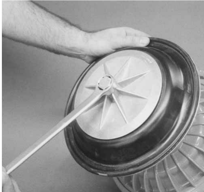
Step 8. Figure 8 Using a 25 mm (1") box wrench, adjustable wrench, or by rotating the diaphragm by hand, remove the diaphragm assembly.
