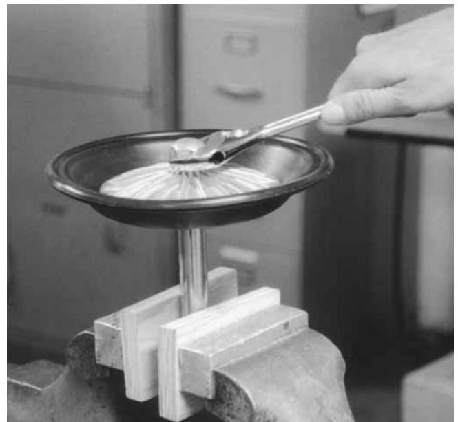
Step 10. Figure 10 To remove the diaphragm assembly from the shaft, secure shaft with soft jaws (a vise fitted with plywood or other suitable material) to ensure shaft is not nicked, scratched, or gouged. Using an adjustable wrench, remove diaphragm assembly from shaft. Inspect all parts for wear and replace with genuine Wilden parts if necessary.
